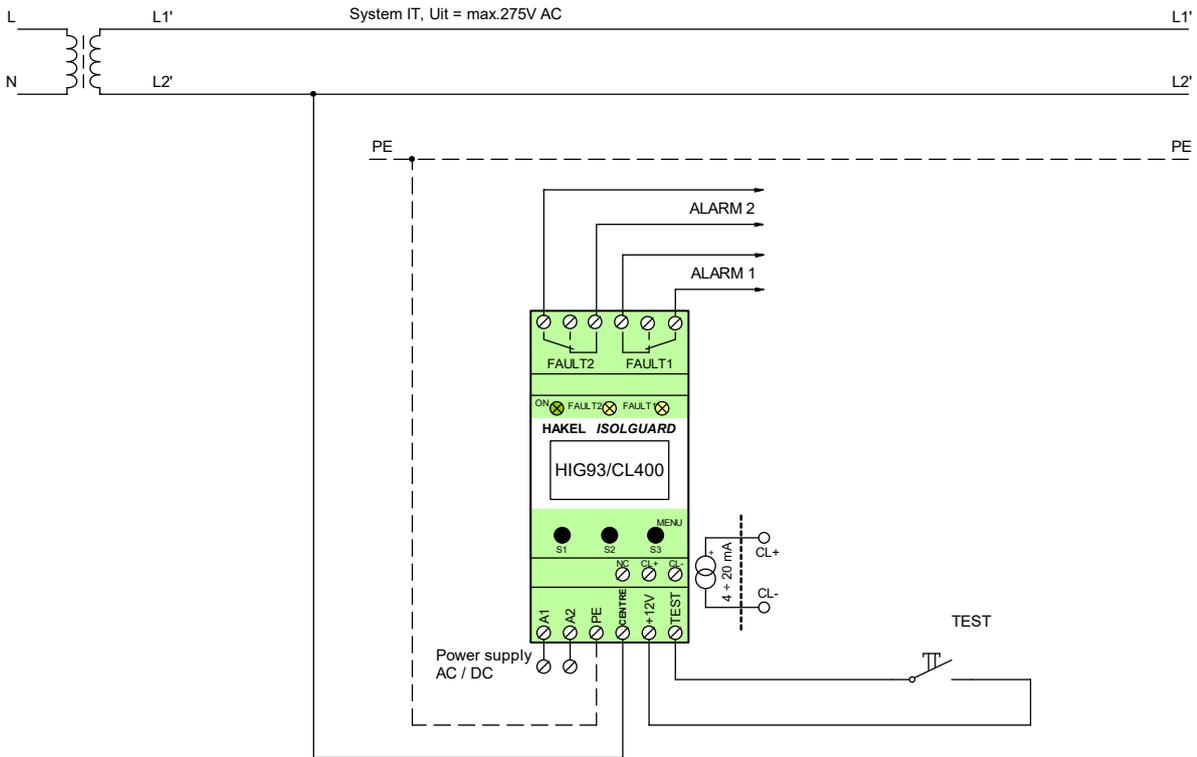
Three-phase IT system (3 x 440 VAC), HIG93/CL400 module with alarm signalling and with the remote test push-button
