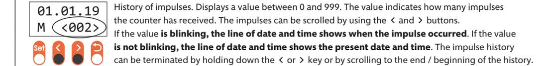
Main menu. By using the < and > buttons to scroll through the menu items. Use the **Set** button to choose the selected menu. Press ↵ to return to the main screen.
